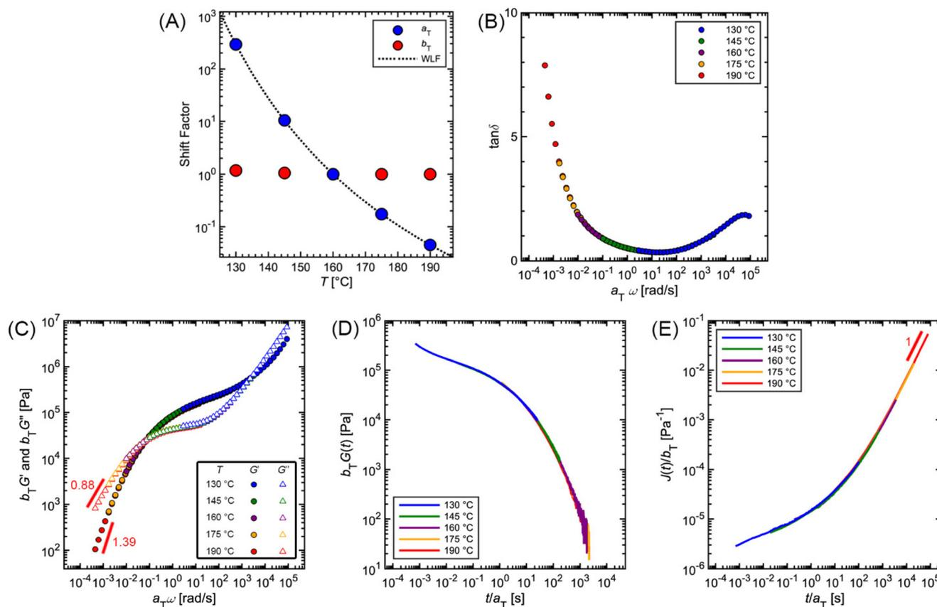
**Fig. 12** Commercial polystyrene time–temperature superposition using  $T_{\text{ref}} = 160$  °C. (A)  $a_T$  and  $b_T$  shift factors. The WLF equation is fit to the experimental  $a_T$  values. (B)  $\tan \delta$ , (C)  $G'$  and  $G''$  (D)  $G(t)$ , and (E)  $J(t)$  master curves.
