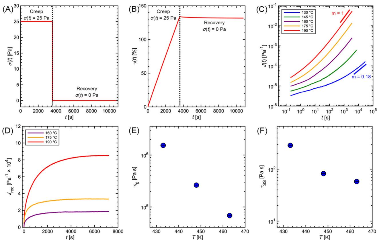
**Fig. 8** Commercial polystyrene creep and recovery measurement. (A) Applied stress and (B) measured strain profiles during creep and recovery. (C) Creep and (D) recoverable compliance versus time. (E) Zero-shear viscosity and (F) steady-state relaxation time versus temperature.
