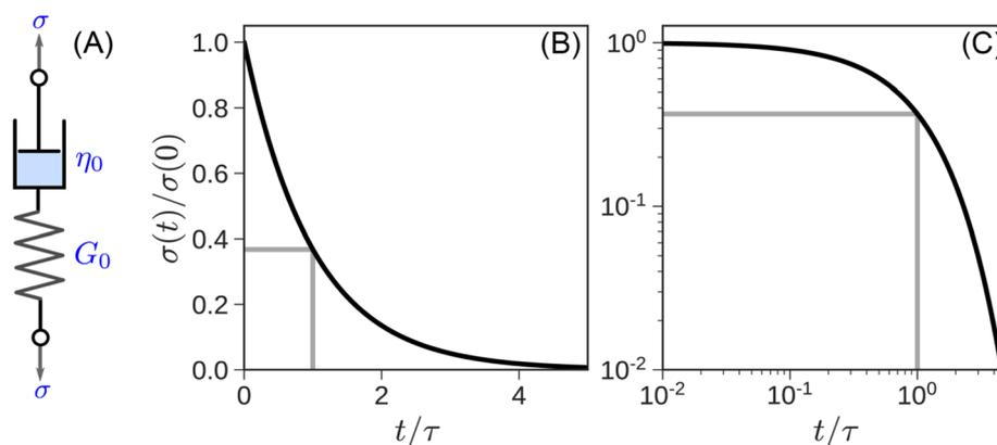
**Fig. 4** (A) A Maxwell element consists of a spring and dashpot in series. (B) Linear–linear and (C) log–log axes plots of the stress relaxation of a Maxwell element subjected to step strain. The gray lines mark the location  $t = \tau$  where the stress falls to  $1/e$  of its initial value, *i.e.*,  $\sigma(t) = \sigma(0)/e$ .
