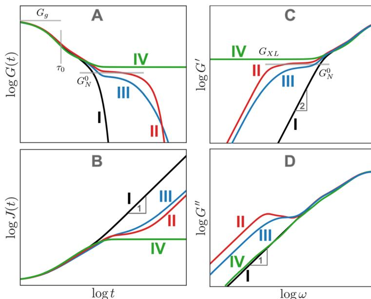
**Fig. 13** Schematic for the (A) stress relaxation modulus, (B) creep compliance, (C) storage and (D) loss moduli of typical polymeric systems: (I) unentangled melt, (II) entangled melt, (III) polydisperse melt, and (IV) permanently cross-linked rubber.
