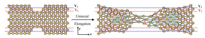
Fig. 3 Schematic of the uniaxial elongation of the PGPN array at a constant pulling velocity  $u = 0.001u_0$  in the x direction. The snapshot of the deformed array is provided at an elongational strain of  $\alpha = 0.6$ . The horizontal dashed blue and red lines demarcate the regions  $Y_1$  and  $Y_2$ , which are normal to the direction of elongation (y direction), respectively. The number of PGPNs within the demarcated regions evolves with strain.
