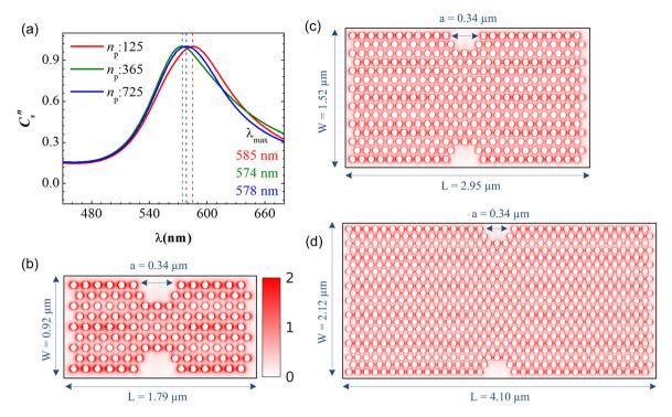
Fig. 2 (a) Normalized scattering cross section,  $C_n^n$ , as a function of wavelength for three PGPN arrays composed of 125 (red curve), 365 (green curve) and 725 (blue curve) PGPNs. Electric field amplitude on the xy-plane (where z = 0) for the arrays with (b) 125, (c) 365 and (d) 725 PGPNs. The structure is illuminated with an X-polarized plane wave propagating in the z direction. The electric field maps are calculated at the resonance wavelengths,  $\lambda_{\text{max}}$ .
