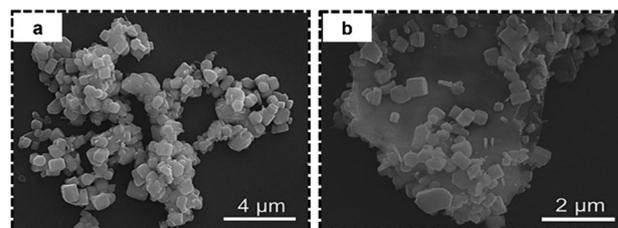
Fig. 26 SEM image of (a)  $\text{Cs}_2\text{AgBiI}_6$  showing agglomerated particles and (b)  $\text{GO}/\text{Cs}_2\text{AgBiI}_6$  showing less agglomerated particles. Reprinted with permission from ref. 138 Copyright 2023, Elsevier.
