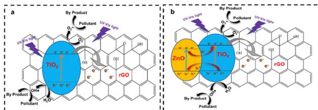
Fig. 19 (a) Illustration of the mechanism of binary-based rGO/TiO<sub>2</sub> as a photocatalyst. (b) Illustration of the mechanism of ternary Z-scheme heterojunction ZnO/rGO/TiO<sub>2</sub>.
