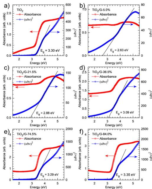
Fig. 23 UV-vis diffuse reflectance spectra and related Tauc plots of  $\text{TiO}_2$  (a) and  $\text{TiO}_2$ /graphene with varying  $\text{TiO}_2$  loadings (5% (b), 21.5 (c), 36.5% (d), 74.5% (e), and 84% (f)). Reprinted with permission from ref. 131 Copyright 2021, Elsevier.
