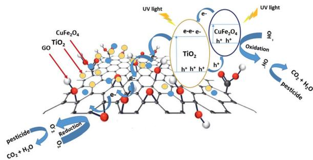
Fig. 24 Proposed mechanism describing the process of charge separation in  $\text{TiO}_2/\text{GO}/\text{CuFe}_2\text{O}_4$  through a direct Z-type scheme when exposed to UV light. Reprinted with permission from ref. 132 Copyright 2020, The Royal Society of Chemistry.
