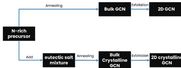
Fig. 3 GCN and crystalline GCN synthesis process.
