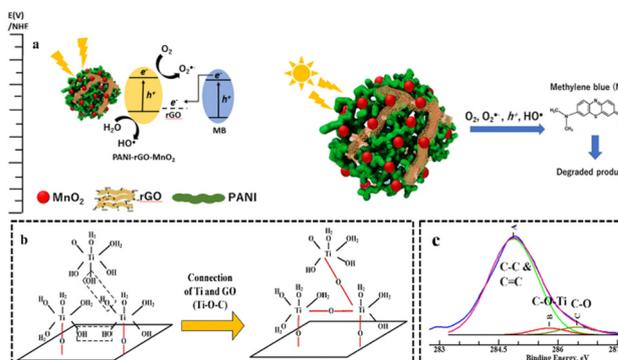
Fig. 27 (a) Schematic illustration of the photocatalytic reduction of MB. Reprinted with permission from ref. 139 Copyright 2019, Elsevier. (b) Illustration of the mechanism of  $\text{TiO}_2$  on the surface of GO sheet. (c) XPS spectra of  $\text{TiO}_2$ -graphene. Reprinted with permission from ref. 140 Copyright 2020, Elsevier.
