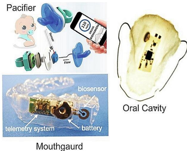
Fig. 9 Wireless embedded sensors for the oral cavity to sense salivary biomarkers *in vivo*. Adapted and reprinted with permissions<sup>164</sup> Copyright (2015), with permission from Elsevier.
