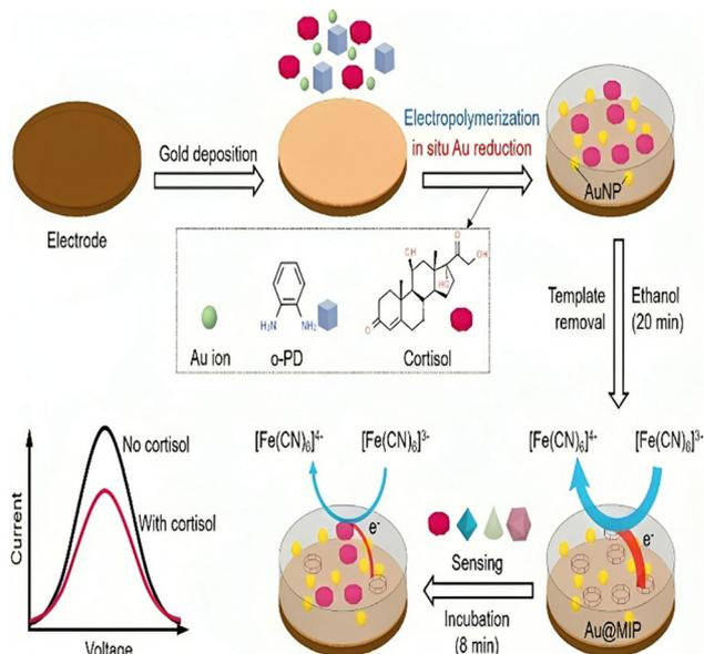
Fig. 7 Fabrication process and sensing mechanism of a cortisol sensor on gold doped MIP layer. Adapted and reprinted with permissions<sup>135</sup> Copyright (2015), with permission from Elsevier.
