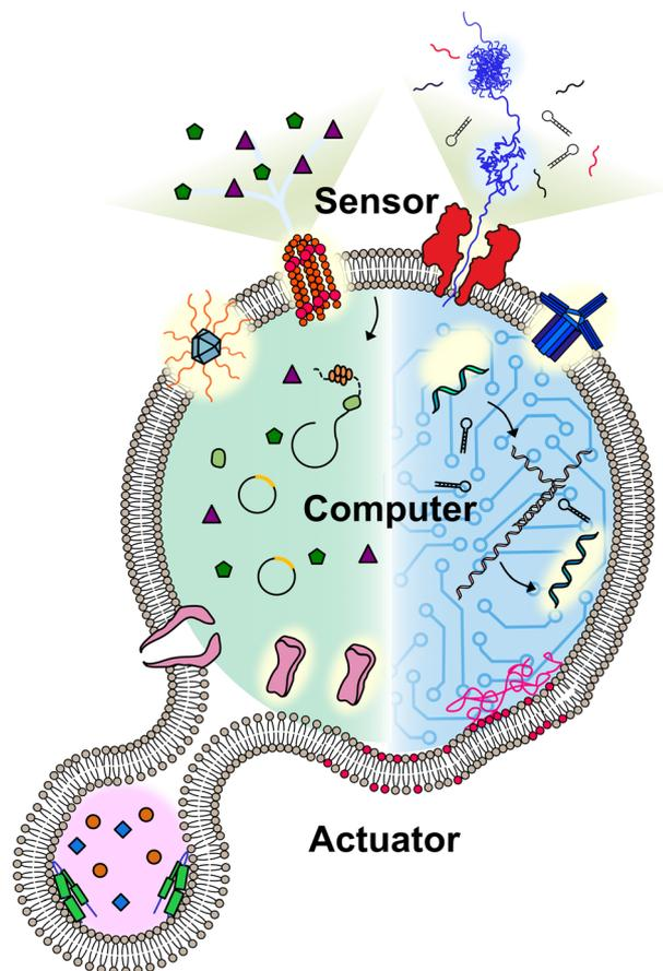
**Fig. 1** Conceptual illustration of a molecular robot including: a body to encapsulate molecular machinery, sensors to collect signals, computers to make decisions, and actuators to perform the tasks.
