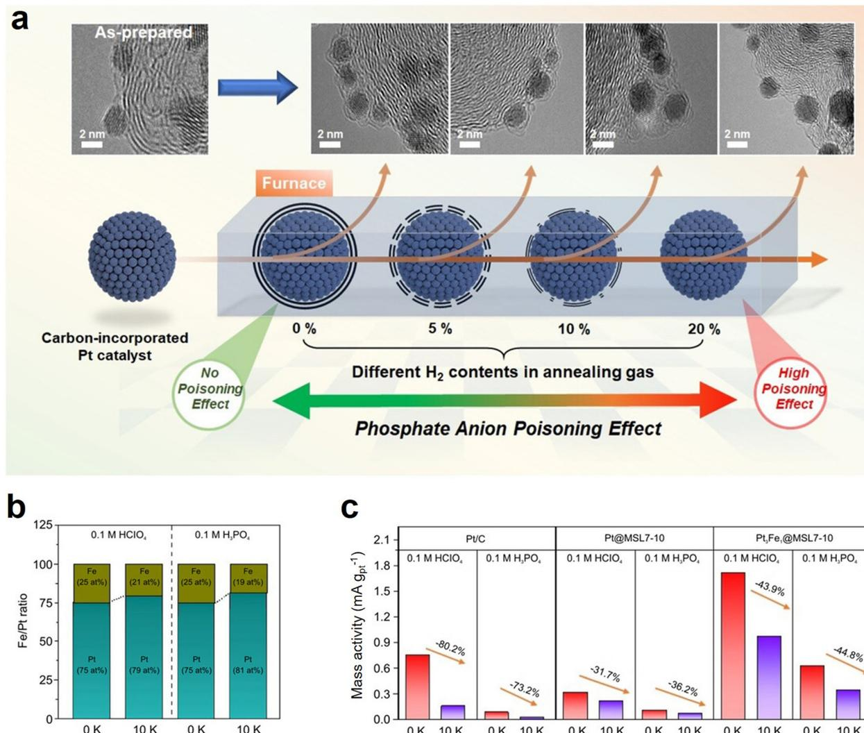
**Fig. 8** (a) Schematic diagram showing the strategy to control the carbon shell structure of Pt-based nanoparticles for realizing the molecular sieve layer effect; (b) Pt/Fe ratios of Pt<sub>3</sub>Fe<sub>1</sub>@MSL7-10 after ADTs; (c) changes in the mass activity of catalysts before and after ADTs. Reprinted with permission from ref. 48. Copyright 2023, John Wiley & Sons.
