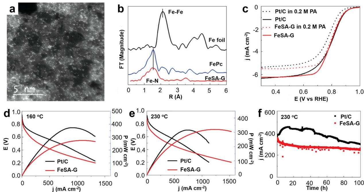
**Fig. 14** (a) AC-STEM images for FeSA-G; (b) Fourier transform of the EXAFS spectra of FeSA-G, FePc, and Fe foil; (c) linear scan voltammetry of FeSA-G and Pt/C;  $J$ - $V$  and power density curves of high temperature PEMFCs at (d) 160 °C and (e) 230 °C; (f) stability of the cells at 0.5 V. Reprinted with permission from ref. 70. Copyright 2019, John Wiley & Sons.
