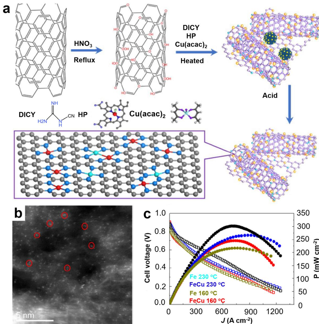
**Fig. 13** (a) Scheme for FeCu-N-CNTs synthesis; (b) AC-STEM; (c) polarization and power density curves of PA/PBI composite membrane cells using FeCu(1:0) and FeCu(4:1) cathodes at 160 and 230 °C. Reprinted with permission from ref. 69. Copyright 2021, Royal Society of Chemistry.
