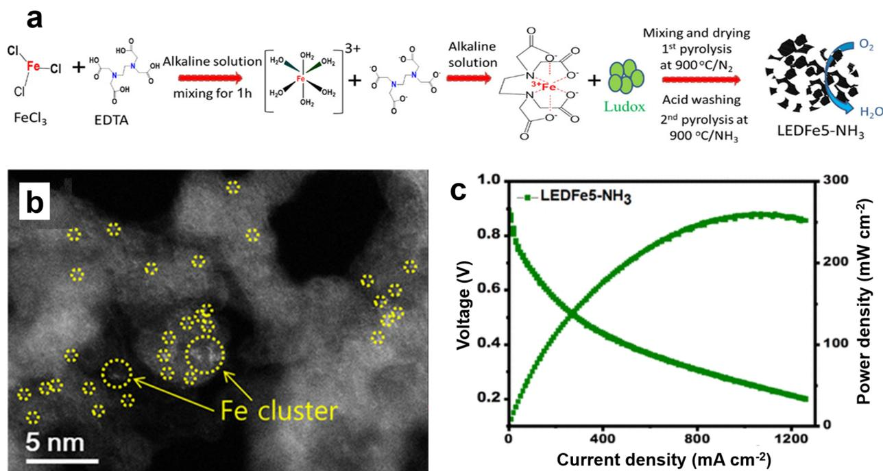
Fig. 12 (a) Schematic illustration of synthesis process for EDTA–Fe complex-based catalyst; (b) HAADF-STEM image of LEDFe<sub>5</sub>-NH<sub>3</sub>; (c) single-cell performance of HT-PEMFC at 1.5 bar O<sub>2</sub> pressure and 150 °C cell temperature. Reprinted with permission from ref. 62. Copyright 2014, American Chemical Society.
