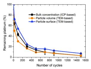
Fig. 5 Comparison of evolution of remaining platinum rate on the electrode as a function of the number of cycles estimated with three different methods: (i) from ICP measurements (black), (ii) from averaged particle volume (orange) and (iii) from averaged surface of particles (deep blue).
