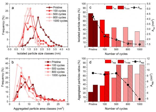
Fig. 2 Distribution of particle (a) diameter for isolated particles and (b) area for aggregated particles; parameters and average area for (c) isolated particles  $r_{n,iso}$  and  $r_{A,iso}$  and (d) aggregated particles  $r_{n,agg}$  and  $r_{A,agg}$  are measured from pristine to 1000 cycles. These parameters are evaluated at different stages of the cycling protocol between 0.4 and 1.2 V vs. RHE in 1 M H<sub>2</sub>SO<sub>4</sub> + 0.01 M NaCl.
