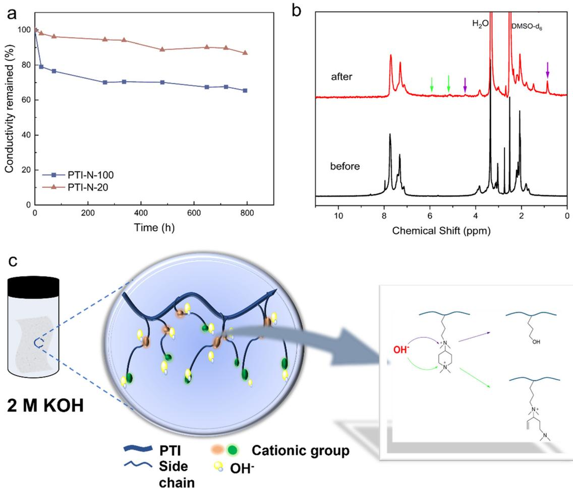
Fig. 8 (a) Curves of ionic conductivity retention versus immersion time of the membranes in 2 M KOH at 80 °C; (b) <sup>1</sup>H NMR of PTI-N-100 membranes after alkali stability testing and (c) schematic diagram of degradation mechanism.
