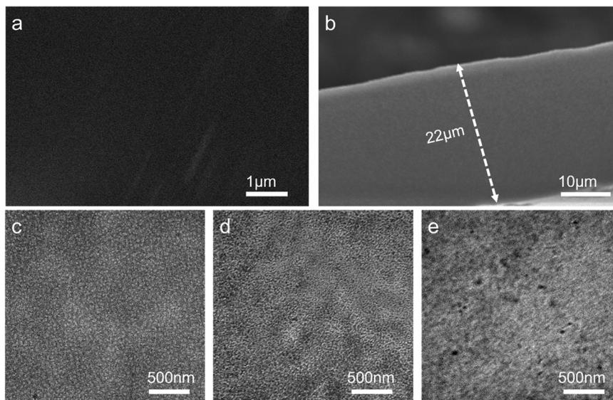
Fig. 4 (a) Surface and (b) cross-sectional SEM images of the PTI-N-100 membrane; TEM images of (c) PTI-N-20, (d) PTI-N-60 and (e) PTI-N-100 membranes, respectively.
