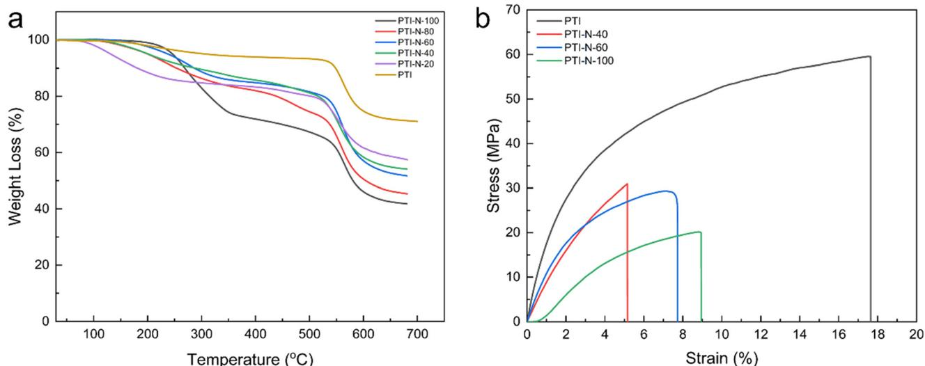
Fig. 7 The graphs of (a) TGA curves of PTI-N-*n* membranes; (b) stress-strain curves of PTI-N-*n* membranes.
