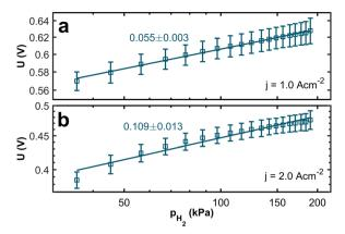
Fig. 3 Logarithmic plot of the voltage at a current density of (a) 1.0 A cm<sup>-2</sup> and (b) 2.0 A cm<sup>-2</sup> against the hydrogen partial pressure. The lines serve as a guide for the eye.
