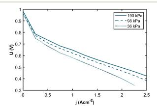
Fig. 2 Polarization curves for partial hydrogen pressures of 190 kPa (solid curve), 98 kPa (dashed curve), and 36 kPa (dotted curve). At 36 kPa, the maximum current density of 2.5 A cm<sup>-2</sup> was not achieved without the cell voltage dropping below 0.3 V, which was specified as the lower voltage limit to ensure low degradation.
