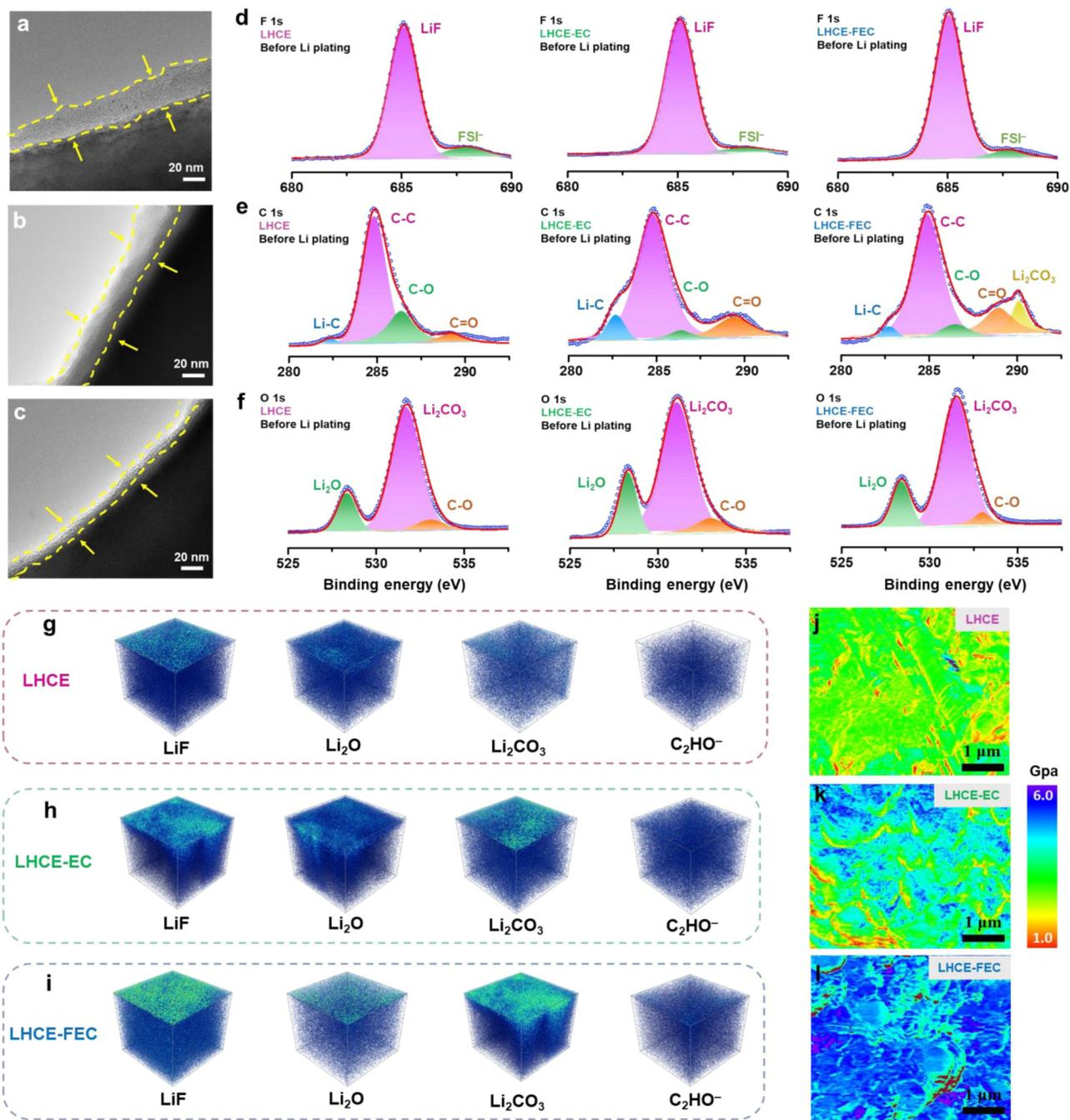
**Fig. 3** TEM images of the SEI before Li plating on the HC anode using (a) LHCE, (b) LHCE-EC, and (c) LHCE-FEC. The surface XPS spectra of (d) F 1s, (e) C 1s, and (f) O 1s on HC anodes using LHCE, LHCE-EC, and LHCE-FEC before Li plating at 0 nm depth, respectively. TOF-SIMS 3D reconstruction models of SEI components formed in (g) LHCE, (h) LHCE-EC, and (i) LHCE-FEC. Young's modulus of the SEI formed in (j) LHCE, (k) LHCE-EC, and (l) LHCE-FEC.
