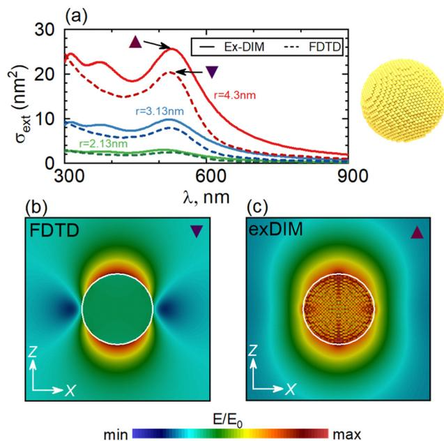
**Fig. 15** Extinction cross section spectra for spherical Au nanoparticles of different sizes in aqueous medium calculated by the Ex-DIM (solid lines) and by the FDTD method (dashed lines) (a); configuration of local electric field calculated for spherical particles with  $r = 4.3$  nm using the FDTD method (b) and Ex-DIM (c) for Au spherical particles at the wavelength  $\lambda = 525$  nm. From ref. 152.
