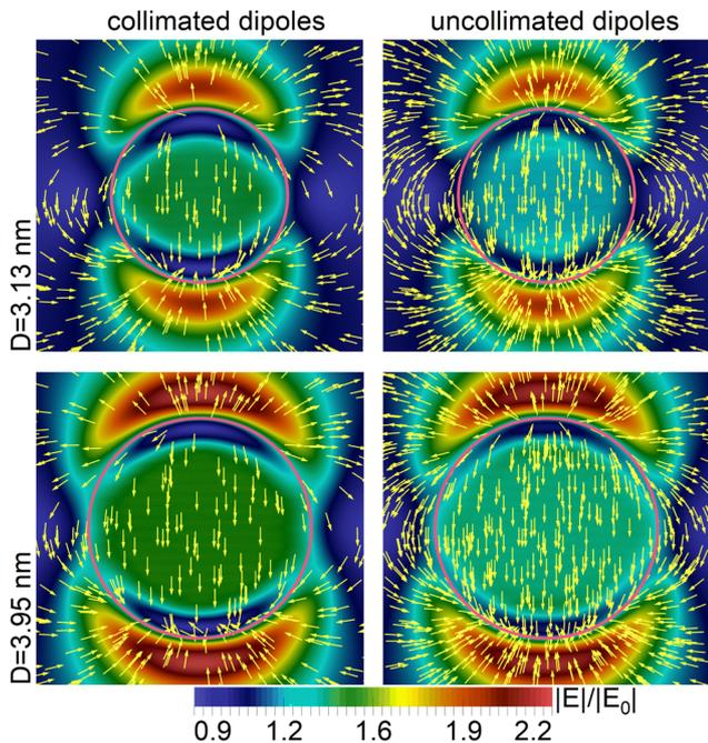
Fig. 19 The maximum field strength modulus and the field direction inside and around the Au nanoparticles with diameter 3.13 and 3.95 nm in than aqueous medium with refractive index  $n = 1.33$  at the wavelength of SPR. On the left: All dipoles in a particle are collimated; on the right: non-collimated dipoles. Polarization is vertical. From ref. 160.
