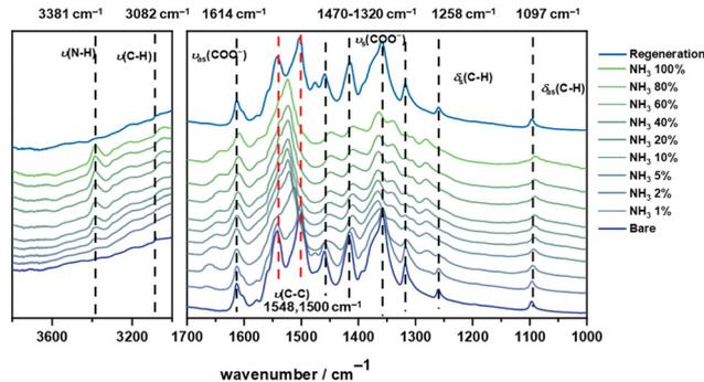
**Fig. 3** *In situ* synchrotron FT-IR spectra of MFM-300(Ti) as a function of  $\text{NH}_3$  adsorption and of regenerated MFM-300(Ti) under a flow of dry  $\text{N}_2$  at  $100\text{ mL min}^{-1}$  at 298 K for 2 h.
