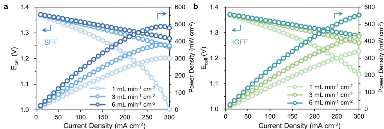
Fig. 6 The polarization curves of (a) SFF-based VRFBs and (b) IGFF-based VRFBs.
