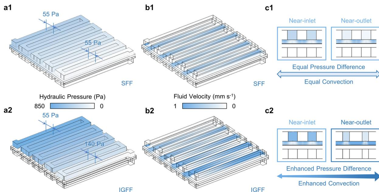
Fig. 3 The (a) hydraulic pressure within flow channels, (b) fluid velocities within porous electrodes and (c) in the cross-view for SFF and IGFF-based batteries.
