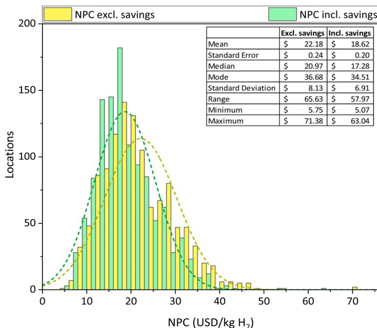
Fig. 5 Histograms of the NPC of H<sub>2,g</sub> “today”, excluding (yellow) and including (green) the potential savings from the sale of surplus electricity. The sale of this electricity would result in an average saving of 11% on the NPC of green H<sub>2</sub>.
