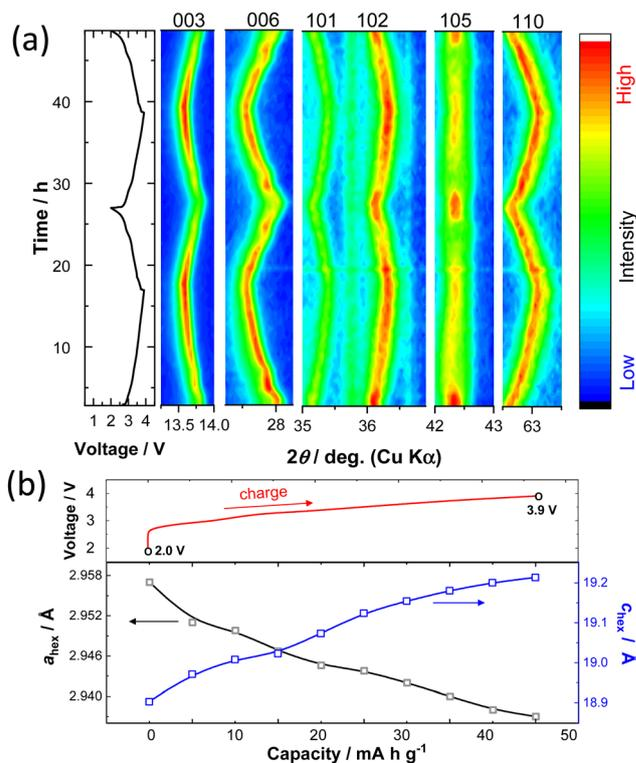
**Fig. 3** Structural changes of  $\text{K}_{0.6-y}\text{Cr}_{0.6}\text{Ti}_{0.4}\text{O}_2$  during charge/discharge; (a) the contour plots of *in situ* XRD data during the first two cycles in the voltage range of 2.0–3.9 V at a rate of  $4 \text{ mA g}^{-1}$ . The voltage change of the *in situ* cell is also shown. (b) Lattice parameter variations during the 2nd charge cycle.
