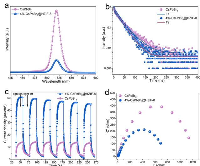
Fig. 5 (a) Steady-state PL spectra of samples. (b) Time-resolved PL decay plots of samples. (c) Photocurrent measurements of samples under visible light illumination ( $\lambda > 420$  nm). (d) Electrochemical impedance measurements of samples.
