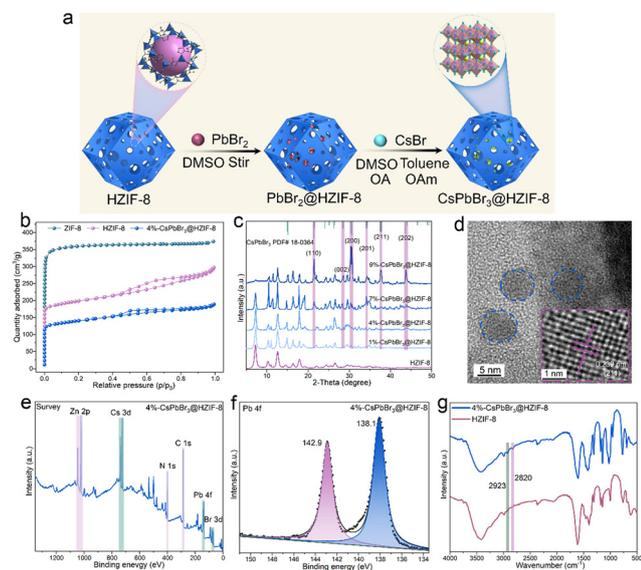
**Fig. 1** (a) Schematic showing the synthesis of CsPbBr<sub>3</sub>@HZIF-8. (b) N<sub>2</sub> adsorption-desorption isotherms of ZIF-8, HZIF-8, and 4%-CsPbBr<sub>3</sub>@HZIF-8 at 77 K. (c) PXRD patterns of samples. (d) TEM and HRTEM images of 4%-CsPbBr<sub>3</sub>@HZIF-8, the lattice fringe of CsPbBr<sub>3</sub>. XPS analysis of samples: (e) survey spectra and (f) Pb 4f spectra. (g) FTIR spectra HZIF-8 and 4%-CsPbBr<sub>3</sub>@HZIF-8.
