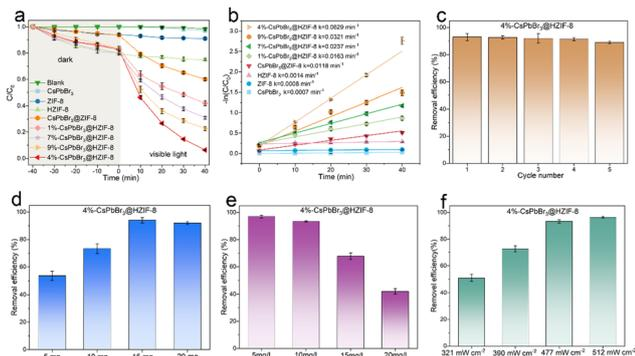
Fig. 3 (a) TCH ( $10 \text{ mg L}^{-1}$ ,  $30 \text{ mL}$ ) degradation dynamics curves and (b) the pseudo-first-order kinetics of TCH degradation over the as-fabricated photocatalysts ( $15 \text{ mg}$ ) under visible light. (c) The recycling performance of 4%-CsPbBr<sub>3</sub>@HZIF-8 for TCH degradation. Impacts of (d) catalyst dosage, (e) TCH concentration and (f) light intensity on TCH photodegradation performance by 4%-CsPbBr<sub>3</sub>@HZIF-8.
