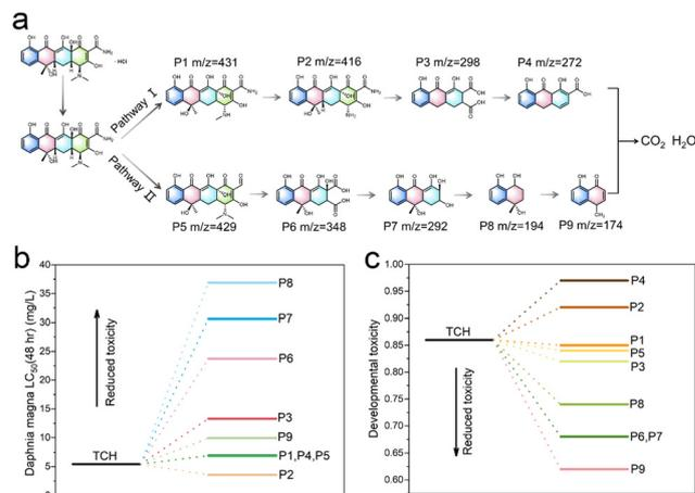
Fig. 6 Possible degradation pathways of TCH in the CsPbBr<sub>3</sub>@HZIF-8 system. Toxicity assessment (b) *Daphnia magna* LC<sub>50</sub> (48 h), and (c) developmental toxicity.
