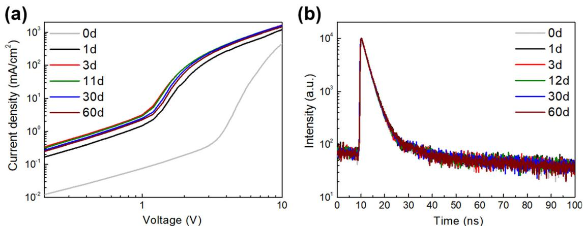
Fig. 2 (a)  $J$ - $V$  curves of the encapsulated electron-only devices with structure ITO/ZnO sol-gel/B-QDs/ZnMgO/Al stored for different days in a nitrogen-filled glovebox. (b) TRPL decay curves of glass/B-QDs/ZnMgO/Al with encapsulation stored for different days in a nitrogen-filled glovebox.
