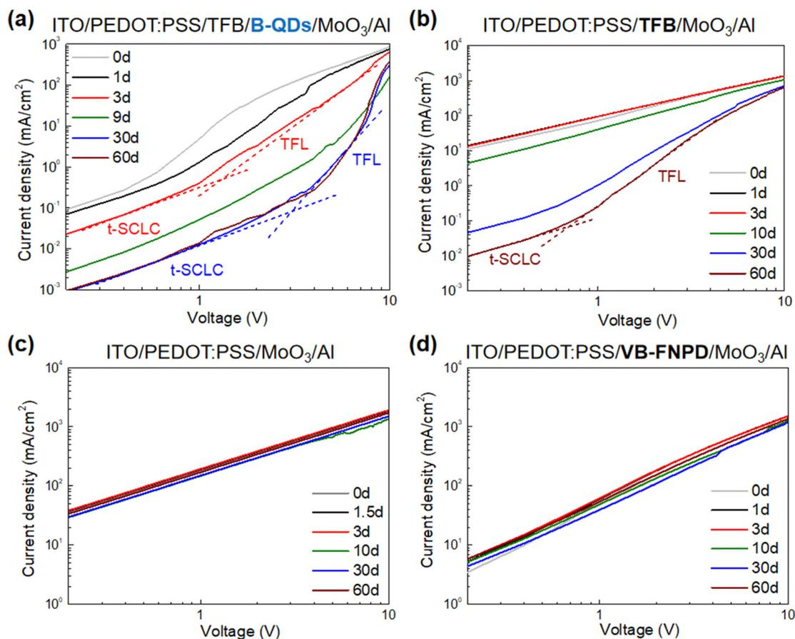
Fig. 3  $J$ - $V$  curves of encapsulated hole-only devices with different structures measured after different storage times in a nitrogen-filled glovebox. (a) ITO/PEDOT:PSS/TFB/B-QDs/MoO<sub>3</sub>/Al (QDs-HODs), (b) ITO/PEDOT:PSS/TFB/MoO<sub>3</sub>/Al (TFB-HODs), (c) ITO/PEDOT:PSS/MoO<sub>3</sub>/Al (PEDOT:PSS-HODs), (d) ITO/PEDOT:PSS/VB-FNPD/MoO<sub>3</sub>/Al (VB-FNPD-HODs).
