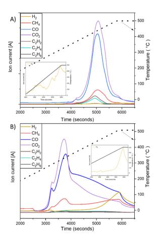
Fig. 2 Gas evolution profile for catalytic pyrolysis experiment (with zoom of  $H_2$  evolution). (A) PET and (B) cotton.
