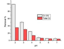
Fig. 3 Removal percentages of Cr(vi) and total chromium that remains in solution for experiments performed with an initial Cr(vi) concentration of 20 ppm; contact time: 24 hours; 1 g  $L^{-1}$  of HMW.
