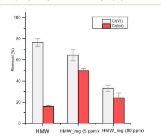
Fig. 7 Reduction of Cr(vi) by HMW and two regenerated lignins, HMW\_reg\_5 and HMW\_reg\_80. pH 2 obtained with 2 M HNO<sub>3</sub>;  $1 \text{ g L}^{-1}$  of lignin; initial Cr(vi) concentration: 5 mg L<sup>-1</sup>; contact time: 2 h.
