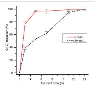
Fig. 6 Influence of contact time on the Cr(vi) reduction. The red line refers to experiments with an initial Cr(vi) concentration of 5 mg L $^{-1}$ , and the dotted line refers to experiments with an initial Cr(vi) concentration of 20 mg L $^{-1}$  (pH = 2, 1 g L $^{-1}$  of HMW).
