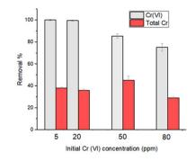
Fig. 5 Removal of chromium(vi) and total chromium after the treatment with  $1 \text{ g L}^{-1}$  of HMW of solutions at different initial concentrations of Cr(vi), and 24 hours contact time at pH 2.
