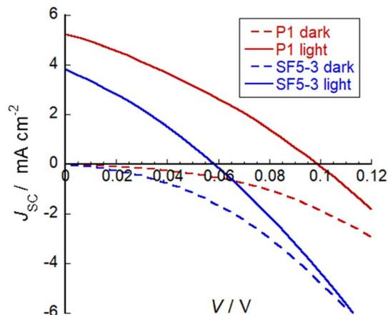
Fig. 7 Plot of current density against voltage for illuminated devices containing dye SF5-3 and the benchmark dye P1. Electrolyte composition: 0.1 M LiI and 1 M I<sub>2</sub> in MeCN.
