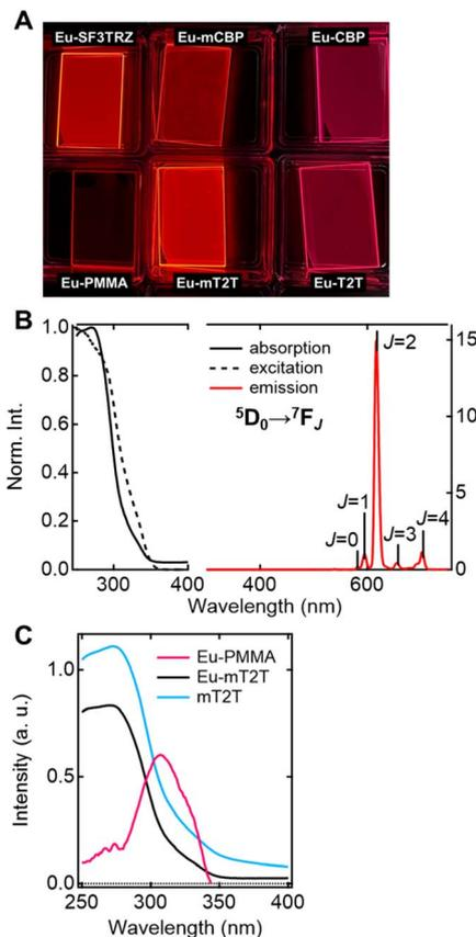
Fig. 3 Optical properties of  $\text{Eu}(\text{hfa})_3(\text{TPPO})_2$ -doped films. (A) Photos of emission from the fabricated films upon photoexcitation with 254 nm. (B) Absorption (solid line), excitation probed at 615 nm (broken line), and emission (red line) spectra of the Eu-mT2T film. (C) Absorption spectra of the Eu-PMMA film (pink line), Eu-mT2T film (black line), and mT2T neat film (sky blue line).
