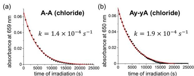
Fig. 6 Decomposition kinetic trace of closed (a) **A-A** and (b) **Ay-yA** under continuous 365 nm light irradiation (112 mW) in water monitored at 659 nm and 650 nm, respectively.
