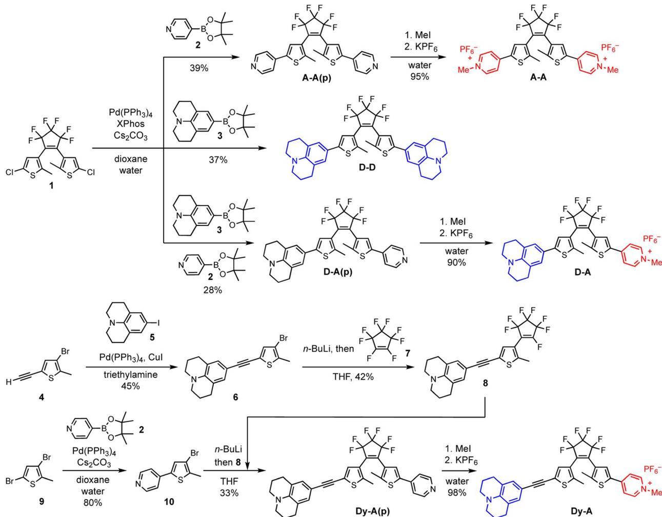
Scheme 2 (Top) Synthesis of D-D, A-A and D-A starting with the construction of DTE dichloride core **1** followed by functionalization of the arm by Suzuki coupling, methylation and ion exchange. **D-A(p)** can be synthesized by Suzuki coupling with two different boronate esters in one pot and then separating the three compounds by column chromatography. (Bottom) Synthetic route to **Dy-A** starting with functionalization of the two arms followed by the construction of DTE core at a later stage.
