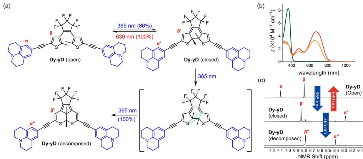
Fig. 7 (a) Proposed decomposition pathway of Dy-yD. (b) Absorption spectra of open-form (blue), closed-form (red), and decomposed product (orange) of Dy-yD recorded in THF. (c) Partial  $^1\text{H}$  NMR spectra of open-form, closed-form, and decomposed product of Dy-yD ( $d_8$ -THF, 500 MHz, 298 K).
