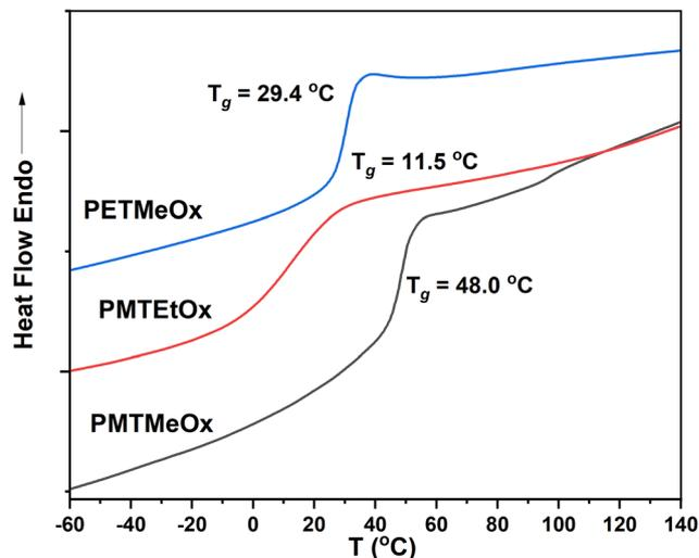
Fig. 3 DSC curves of the homopolymers.
