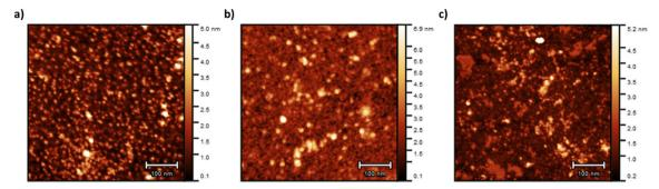
Fig. 4 AFM pictures of (a) Star 1, (b) Star 2 and (c) Star 3. The samples were prepared at 0.025 mg mL<sup>-1</sup> onto freshly cleaved mica
