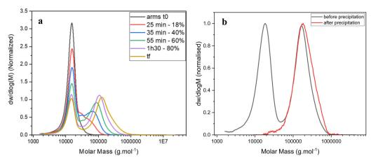
Fig. 2 GPC traces of (a) the kinetic of star formation ([CL] = 0.2 M, [CL]/[mCTA] = 3, [mCTA]/[I] = 20) – samples are taken at 0 minute (t0), 25, 35 55 and 90 minutes and at the end of the reaction (tf – 180 minutes; 95% crosslinker conversion) – the percentage corresponds to the crosslinker conversion measured by <sup>1</sup>H NMR; (b) star poymer at tf and after purification by precipitation, showing complete removal of unreacted arms.
