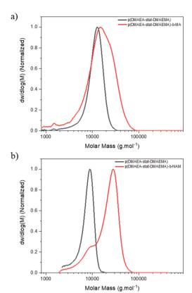
Fig. 1 DMF-GPC chromatogram of chain extension of p(DMAEA-stat-DMAEMA) with (a) MA, (b) NAM.
