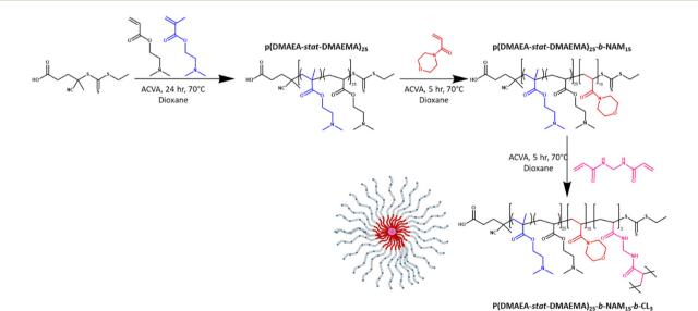
Scheme 1 Synthesis of p(DMAEA-stat-DMAEMA)<sub>25</sub>-b-NAM<sub>15</sub>-b-CL<sub>3</sub> star copolymer by the arm-first approach.
