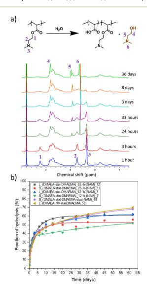
Fig. 5 (a) <sup>1</sup>H NMR spectrum illustrating hydrolysis of DMAEA side chains to release DMAE in D<sub>2</sub>O over 36 days for p(DMAEA-stat-DMAEAMA)<sub>25</sub>-b-NAM<sub>15</sub> linear arms. (b) Hydrolysis kinetics of stars (S) and their corresponding arms (L) in D<sub>2</sub>O over 62 days determined by <sup>1</sup>H NMR spectroscopy.
