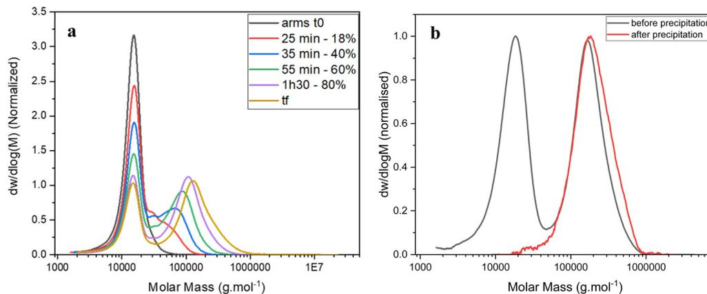
**Fig. 2** GPC traces of (a) the kinetic of star formation ( $[CL] = 0.2$  M,  $[CL]/[mCTA] = 3$ ,  $[mCTA]/[I] = 20$ ) – samples are taken at 0 minute ( $t_0$ ), 25, 35 55 and 90 minutes and at the end of the reaction ( $t_f$  – 180 minutes; 95% crosslinker conversion) – the percentage corresponds to the crosslinker conversion measured by  $^1\text{H}$  NMR; (b) star polymer at  $t_f$  and after purification by precipitation, showing complete removal of unreacted arms.
