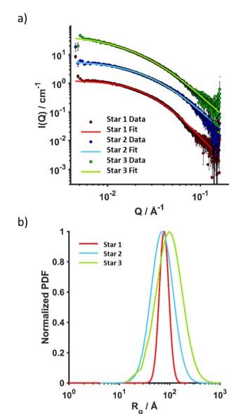
Fig. 3 SAXS analysis in DMF (2 mg mL $^{-1}$ , 25 °C) of Star 1, Star 2 and Star 3. (a) Overlay of raw data and fittings (polydisperse star polymer model), (b) radius of gyration fit to a lognormal distribution.
