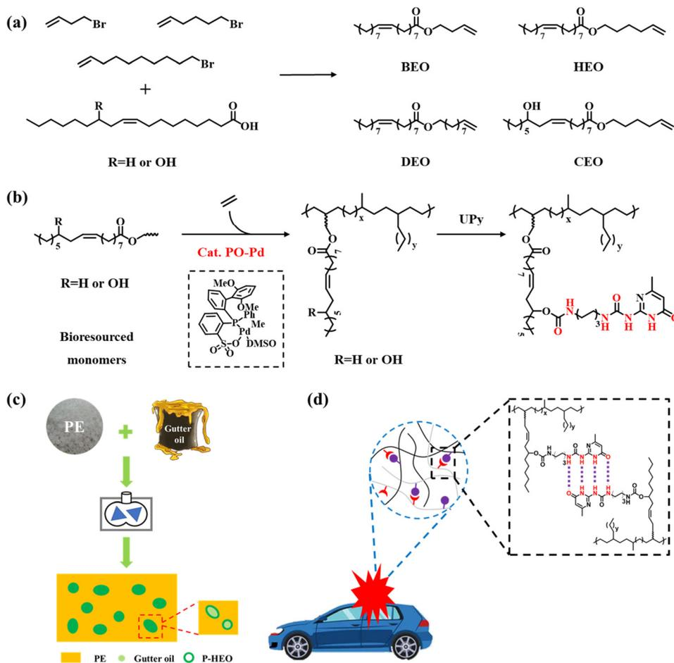
**Scheme 2** (a) Palladium-catalyzed copolymerization of ethylene with a polar comonomer. (b) The bioresourced comonomers copolymerized with ethylene. (c) Schematic diagram of P-HEO toughened HDPE/gutter oil. (d) A polyolefin protective gear schematic with complementary hydrogen bonding interactions.
