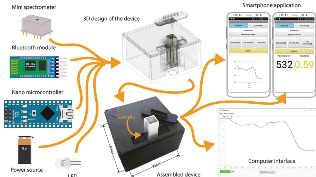
Fig. 8 Portable handheld colorimetric detection of phosphate [this figure has been reproduced from ref. 37 under open access article in terms of the Creative Commons CC-BY license].
