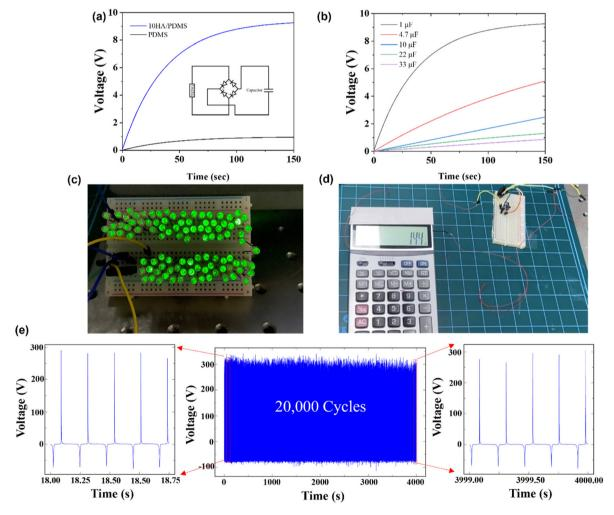
Fig. 5 (a) The charging curves of a 1 µF capacitor comparing PDMS and optimal 10HA/PDMS at an input frequency of 5 Hz and an applied force of 2 N. (b) The charging curves of different capacitors with optimized 10HA/PDMS at an applied force of 2 N. (c and d) HA-TENG powering 100 LEDs or a commercial calculator. (e) Endurance test of the optimized HA-TENG for more than 20 000 cycles.
