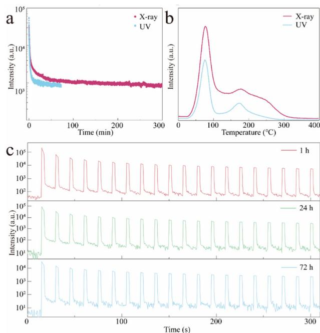
**Fig. 4** (a) Afterglow decay curves, and (b) the TL glow curves of CCCP:2%Mn<sup>2+</sup> after excitation by 254 nm UV light and X-rays for 10 min. (c) The repeated OSL obtained at different decay times (1, 24, and 72 h) with an 870 nm NIR light stimulus. The stimulation time in each cycle was set as 3 s.
