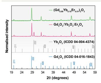
Fig. 1 X-ray diffraction patterns of 1 (green line) and 2 (red line) (powders). The reflections of cubic Gd<sub>2</sub>O<sub>3</sub> and Yb<sub>2</sub>O<sub>3</sub> are also depicted.
