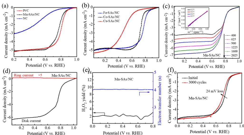
**Fig. 5** ORR performance in 0.5 M  $\text{H}_2\text{SO}_4$  solution. (a and b) LSV curves of various catalysts at a rotating speed of 1600 rpm. (c) LSV curves and K–L plots (the inset) of Mn–SAs/NC at different rotating rates. (d) RRDE measurements of Mn–SAs/NC and (e) the corresponding electron transfer number and  $\text{H}_2\text{O}_2$  yield. (f) The LSV curves before and after the CV cycling test for Mn–SAs/NC.
