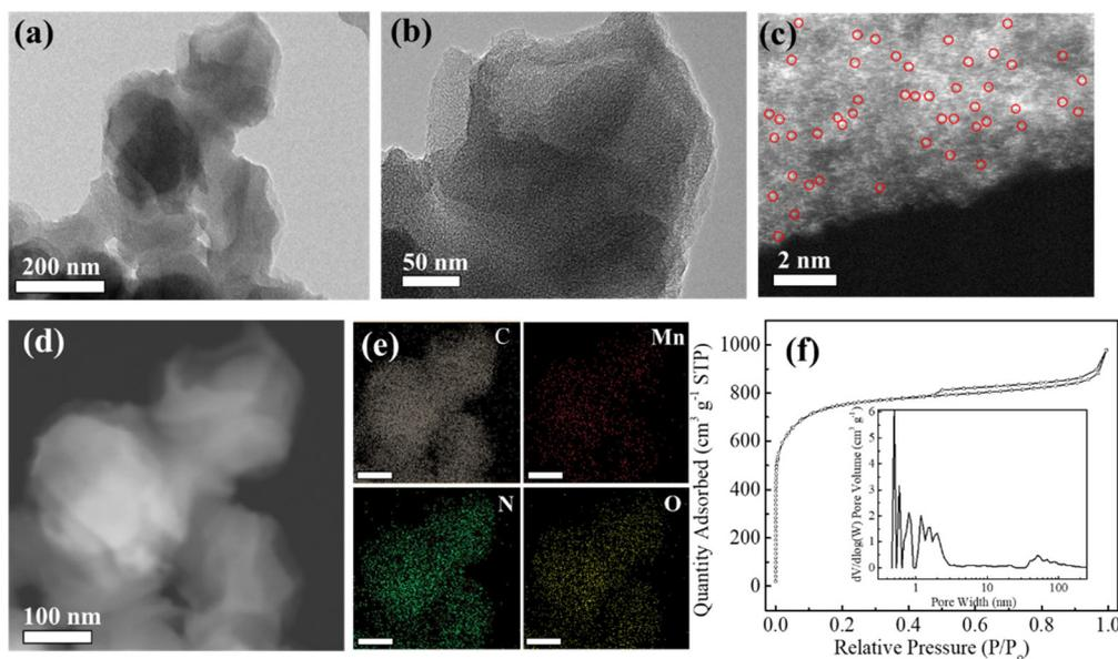
**Fig. 1** (a and b) TEM images at different magnifications of Mn–SAs/NC. (c) Aberration-corrected HAADF-STEM image of Mn–SAs/NC. (d and e) HAADF-STEM image and the corresponding elemental mappings of C, Mn, N, and O elements in Mn–SAs/NC. (f)  $\text{N}_2$  adsorption–desorption isotherms and pore size distribution based on the BJH method (the inset).
