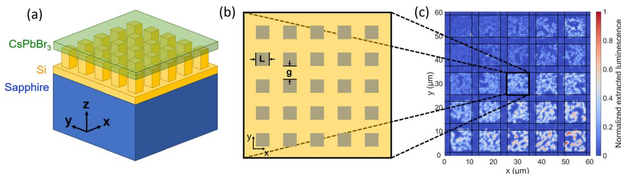
**Fig. 1** (a) Schematic representation of the CsPbBr<sub>3</sub> layer deposited on Mie resonators, each corresponding to a set of  $(L,g)$  parameters. (b) Geometric parameters defining the size of the square pillars ( $L$ ) and their side-to-side separation, which we refer to as the gap ( $g$ ). (c) Perovskite luminescence, normalized to the maximum intensity of the image, over Mie resonators with varying  $(L,g)$  parameters.
