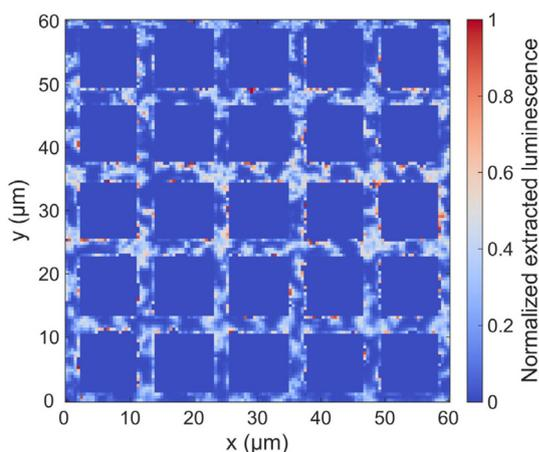
**Fig. 8** Spatially-resolved perovskite luminescence normalized to the maximum intensity of the image on the silicon regions with no pillars, highlighted in Fig. 2b. Note that the PL signal from the perovskite-on-Mie resonators, which is roughly ten to twenty times more intense, has been removed in the current image.
