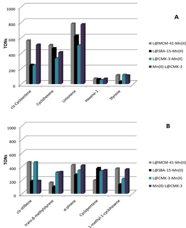
**Fig. 9** (A and B) TOFs for alkene epoxidation catalyzed by L@MCM-41-Mn(II), L@SBA-15-Mn(II), L@CMK-3-Mn(II) and Mn(II)-L@CMK-3 in the presence of  $\text{H}_2\text{O}_2$ . Conditions: [catalyst :  $\text{H}_2\text{O}_2$  :  $\text{CH}_3\text{COONH}_4$  : substrate] = [1 : 2000 : 1000 : 1000]; catalyst = 1 mol in 0.85 mL  $\text{CH}_3\text{COCH}_3$  :  $\text{CH}_3\text{OH}$  (0.45 : 0.40). Reproduced with permission from ref. 202. Copyright 2016, Elsevier B.V.
