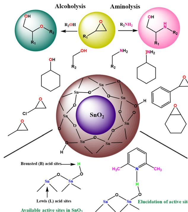
Scheme 3 Alcoholysis and aminolysis of epoxides using tin oxide as the catalyst.
