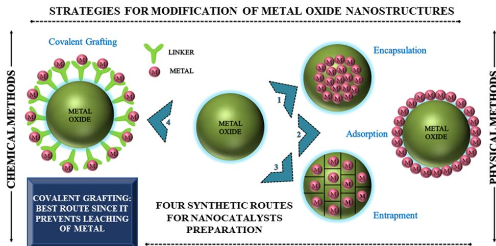
Fig. 4 Strategies for modification of metal oxide nanostructures.
