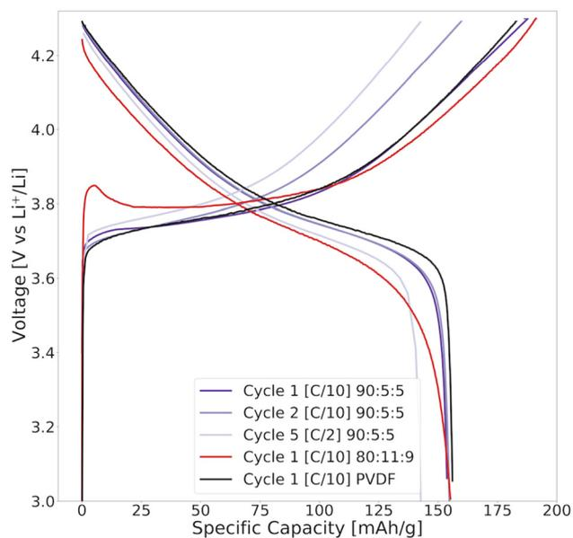
**Fig. 13** The voltage profile of the first and second cycles at C/10 and the fifth cycle at C/2 for NMC111 cathodes fabricated using 80:11:9 (red) or 90:5:5 (purple) lignin/water ( $7.4 \text{ mg cm}^{-2}$ ), and 85:10:5 PVDF/NMP-fabricated cathodes (black) ( $6.9 \text{ mg cm}^{-2}$ ). The cathodes were cycled in coin cells between 3.0 and 4.3 V (vs.  $\text{Li}^+/\text{Li}$ ) at different [C-rates] at 22 °C using a Li metal anode.  $1\text{C} = 160 \text{ mA g}^{-1}$ .
