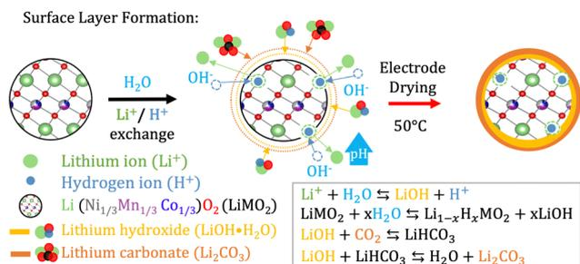
Fig. 2 When the NMC material is exposed to water  $\text{Li}^+$  starts leaching out from its structure while  $\text{H}^+$  from the water intercalates with the structure.<sup>44</sup>  $\text{OH}^-$  in the solution steadily increases the pH and combines with  $\text{Li}^+$  to form LiOH as the water evaporates during electrode drying. Furthermore, LiOH reacts with  $\text{CO}_2$  to form  $\text{LiHCO}_3$  and eventually  $\text{Li}_2\text{CO}_3$ .
