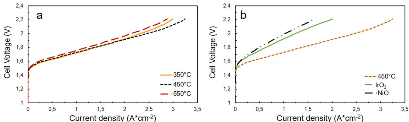
Fig. 6 Comparison of  $I$ - $V$  curves at 60 °C (a) among the differently treated NiFeOx-based cells and (b) among the cells equipped with NiFe-oxide, IrO<sub>2</sub>, and NiO at the anode.
