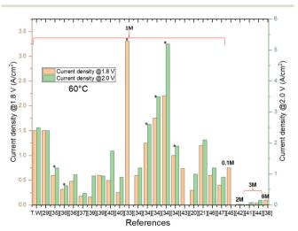
Fig. 7 Comparison at 60  $^{\circ}$ C among the values of current densities from the literature obtained at 1.8 V and 2.0 V, with different KOH concentrations. \* corresponds to cells based on noble metals at both anode and cathode.
