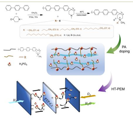
Fig. 7 Synthesis of PTP and fabrication of PTP-Cx membranes
