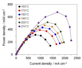
Fig. 6 Unhumidified  $H_2$ -air fuel cell performances of the cell assembled with the PTP-C5/202% PA membrane without backpressure at different temperatures. The Pt catalyst loading in both electrodes was 1.5 mg cm<sup>-2</sup>.
