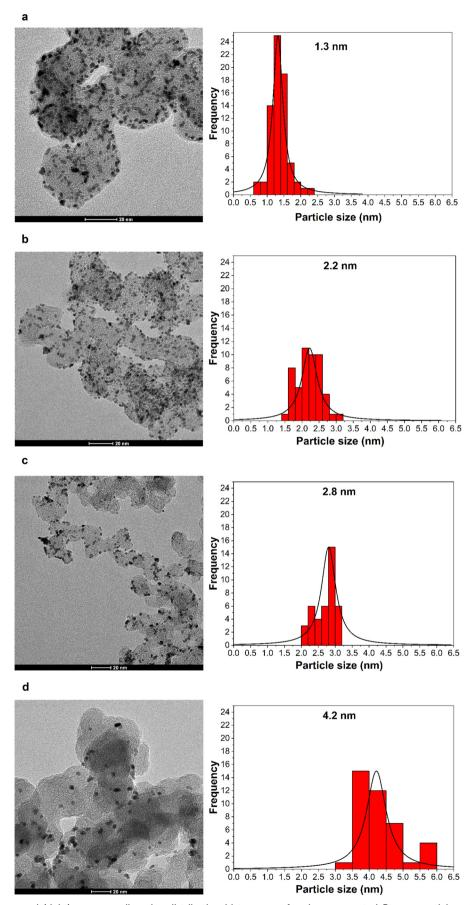
Fig. 1 (Left) TEM images and (right) corresponding size distribution histograms of carbon-supported Pt nanoparticles of various mean particle sizes: - (a) 1.3 nm, (b) 2.2 nm, (c) 2.8 nm, (d) 4.2 nm.
