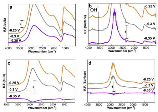
Fig. 7 PM-IRRAS spectra (considering ammonia at -0.5 V as reference) on Pt/C of (a), (b) 1.3 nm size and (c), (d) 2.2 nm particle size during ammonia electro-oxidation in 1 M KOH + 0.5 M NH<sub>4</sub>OH. Spectra collected after 30 min at each potential. The left hand side corresponds to the bulk of the electrolyte and the right hand side corresponds to the Pt surface.
