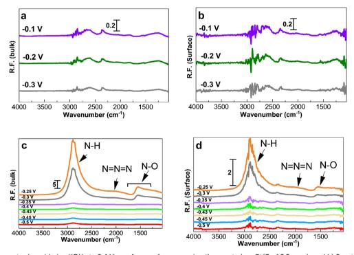
Fig. 6 PM-IRRAS spectra (considering KOH at -0.4 V as reference for processing the spectra) on Pt/C of 2.2 nm. (a and b) Spectra in 1 M KOH and (c and d) spectra in 1 M KOH + 0.5 M NH<sub>4</sub>OH. The applied potentials in (c) and (d), as indicated in the figure, are -0.5, -0.45, -0.45, -0.45, -0.45, -0.45, -0.45, and -0.25 V. The left hand side corresponds to the bulk of the electrolyte and the right hand side corresponds to the Pt surface.
