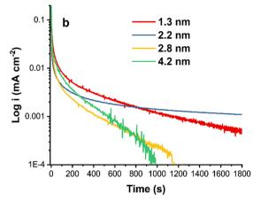
Fig. 3 (a) A comparison of the forward CV scans of Pt/C catalysts at  $v = 20 \text{ mV s}^{-1}$  and (b) chronoamperograms of Pt/C catalysts at -0.3 V in 1 M KOH + 0.5 M NH₄OH.
