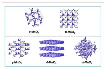
Fig. 4 Crystal structures of  $\alpha$ -MnO<sub>2</sub>,  $\beta$ -MnO<sub>2</sub>,  $\gamma$ -MnO<sub>2</sub>,  $\delta$ -MnO<sub>2</sub>, and λ-MnO<sub>2</sub>. Reprinted with permission from ref. 110. Copyright 2018. Elsevier.
