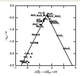
Fig. 3 OER volcano map of transition metal-based oxides. Reprinted with permission from ref. 49. Copyright 2021, Small.
