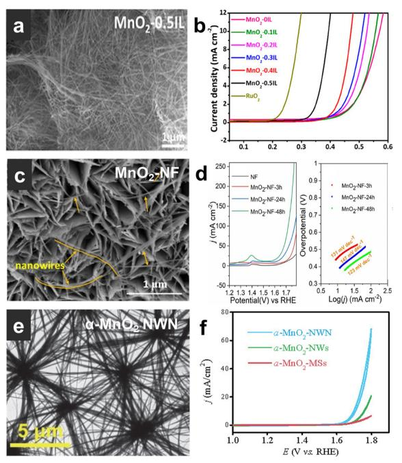
Fig. 5 (a) (c) and (e) TEM images of  $MnO_2$ -0.5IL,  $MnO_2$ -NF, and  $\alpha$ -MnO<sub>2</sub> NWN. (b) (d) and (f) Electrocatalytic OER performance of  $MnO_2$ -0.5IL, MnO<sub>2</sub>-NF, and α-MnO<sub>2</sub> NWN. Reprinted with permission from ref. 85. Copyright 2018, ACS Catal. Reprinted with permission from ref. 59. Copyright 2022, Chem. Eng. J. Reprinted with permission from ref. 86. Copyright 2021, Chin. J. Catal.
