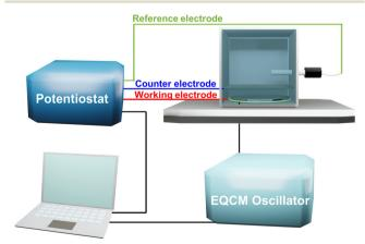
Fig. 2 Scheme of EQCM system.
