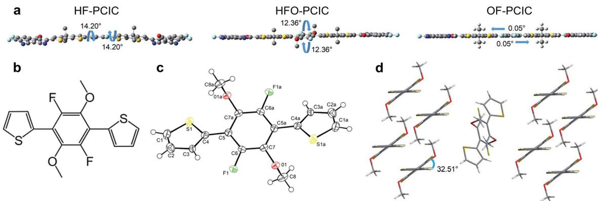
**Fig. 3** (a) Molecular geometries of HF-PCIC, HFO-PCIC and OF-PCIC acceptors. (b) Chemical structure of model compound FPT-O. (c) Single crystal structure of FPT-O. (d) Molecular packing (reprinted with permission from ref. 34 Copyright 2018 The Royal Society of Chemistry).
