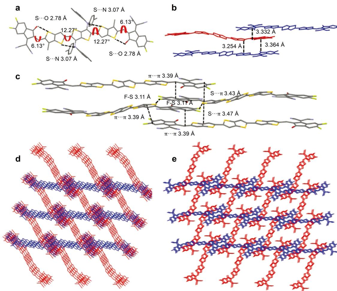
**Fig. 4** (a) The single-crystal structure of 2BTh-2F; (b) the face-to-face distance in the triclinic system; (c) the intermolecular interactions between adjacent molecules; (d) 3D molecular packing along the *b*-crystallographic axis; (e) 3D molecular packing along the *c*-crystallographic axis (reprinted with permission from ref. 29 Copyright 2021 Wiley-VCH).
