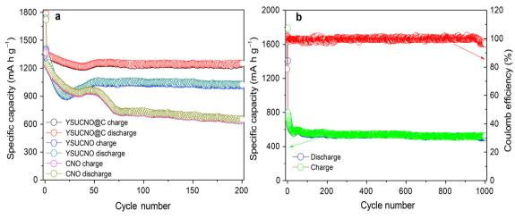
Fig. 3 Cycling stability curves of (a) the YSUCNO, YSUCNO@C, and CNO microspheres at 0.1 C for 200 cycles and (b) the YSUCNO@C microspheres at 5 C for 1000 cycles.
