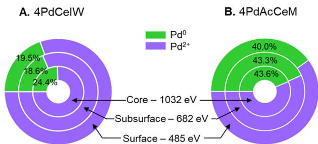
Fig. 3 Comparison of the measured Pd<sup>0</sup>/Pd<sup>2+</sup> amount at different penetration depths on (A) 4PdCeIW and (B) 4PdAcCeM under 0.6 mbar CH<sub>4</sub> and 1.4 mbar O<sub>2</sub> at 873 K.
