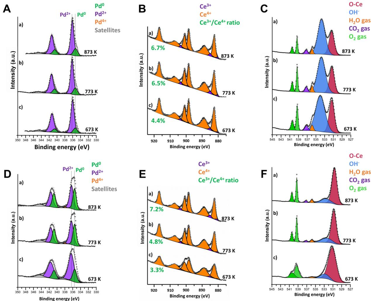
Fig. 2 NAP-XPS spectra collected on 4PdCeIW (A–C) and 4PdAcCeM (D–F) in the Pd 3d (A and D), Ce 3d (B and E) and O 1s (C and F) regions under 0.6 mbar CH<sub>4</sub> and 1.4 mbar O<sub>2</sub> at increasing temperatures: (c) 673 K, (b) 773 K, (a) 873 K.
