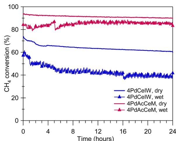
Fig. 5 Methane oxidation activity of 4PdAcCeM and 4PdCeIW under stoichiometric methane oxidation conditions held at 723 K for 24 hours; in a dry atmosphere (solid line) and with 10 vol% H<sub>2</sub>O added to the feed (trace with symbols). Measured CO<sub>2</sub> selectivity on all samples: 100%.
