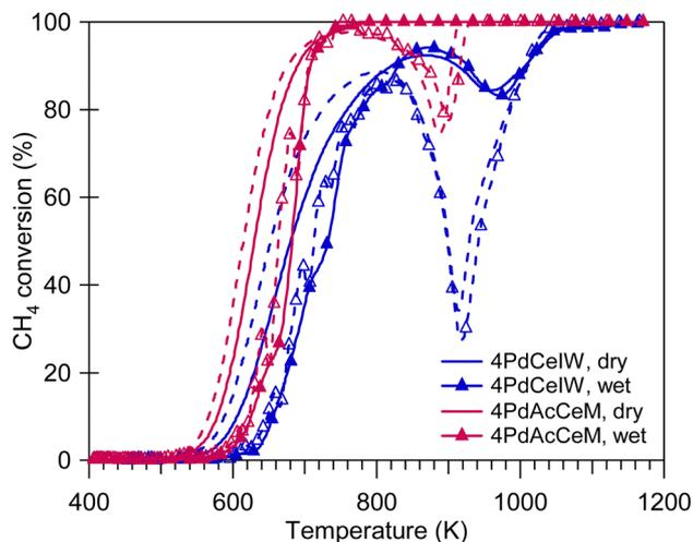
Fig. 4 Methane oxidation activity of 4PdAcCeM and 4PdCeIW under stoichiometric methane oxidation conditions, in a dry atmosphere and with 10 vol% H<sub>2</sub>O added to the feed (wet). Solid line: heating; dashed line: cooling.
