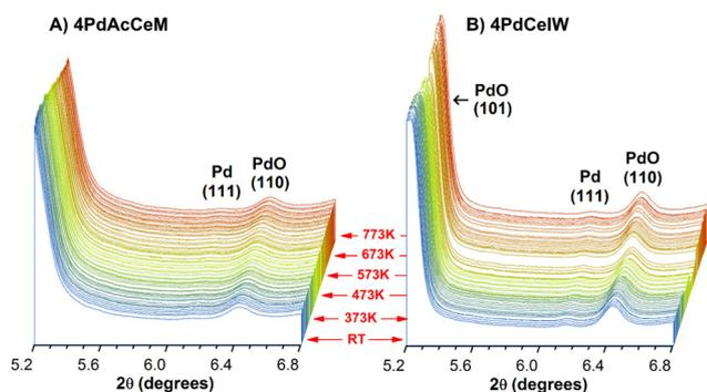
Fig. 1 *In situ* XRD diffraction patterns collected under stoichiometric methane oxidation conditions (0.3% CH<sub>4</sub>, 0.6% O<sub>2</sub> in He) on (A) 4PdAcCeM and (B) 4PdCeIW; samples were heated from RT to 773 K at a 10 K min<sup>−1</sup> heating rate, and scans were collected every 60s.
