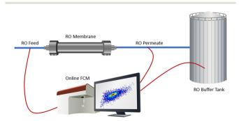
Fig. 1 Simplistic schematic overview of the installation and different sampling points (RO feed, RO permeate  $\theta$  RO tank).
