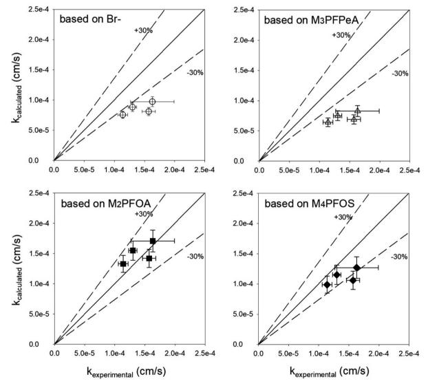
Fig. 4 Comparison of the observed mass transfer coefficient of PFOA, PFHxS, PFOS, and 6:2 FTS (k<sub>experimental</sub>, measured in the experiments presented in Fig. 3) and the mass transfer coefficient ( $k_{\text{calculated}}$ ) calculated based on eqn (3). The solid lines are the 1:1 lines, whereas the dashed lines represent the  $\pm 30\%$  relative percent difference between  $k_{\rm experimental}$  and  $k_{\rm calculated}$
