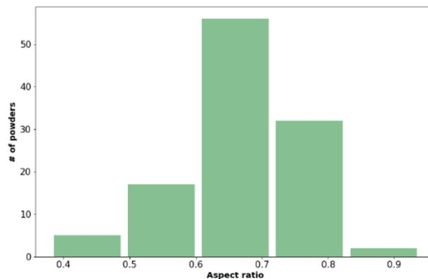
**Fig. 1** The distribution of aspect ratio values across the materials included in the training data set. Values presented here are the mean values from three measurements.
