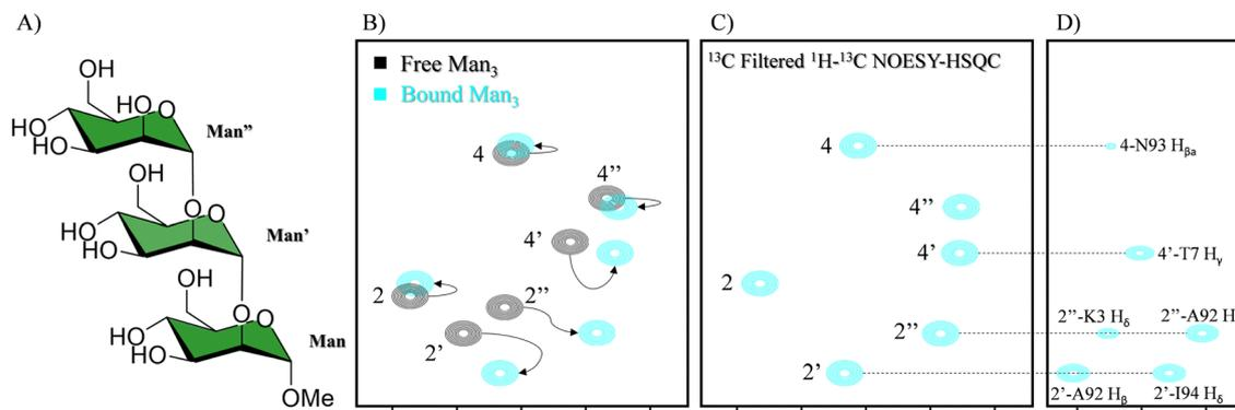
Fig. 22 (A) Scheme of  $\text{Man}_3$ . (B) In black  $^1\text{H}$ - $^{13}\text{C}$  HSQC of the  $^{13}\text{C}$  labelled  $\text{Man}_3$  and in blue in the presence of CV-N. The shift of the signal is indicated with arrows (C) sugar region of the  $^{13}\text{C}$  filtered NOESY-HSQC (D) side chain region of the  $^{13}\text{C}$  filtered NOESY-HSQC. NOEs between the glycan and CV-N are indicated. Adapted from ref. 131.
