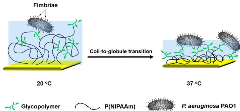
Fig. 16 The adhesion of *P. aeruginosa* to a thermoresponsive polymer coating results in stronger adhesion in the collapsed state of the polymers above the LCST due to an increase in carbohydrate density and hydrophobic interactions. Reprinted with permission from ref. 203 Copyright 2015 American Chemical Society.
