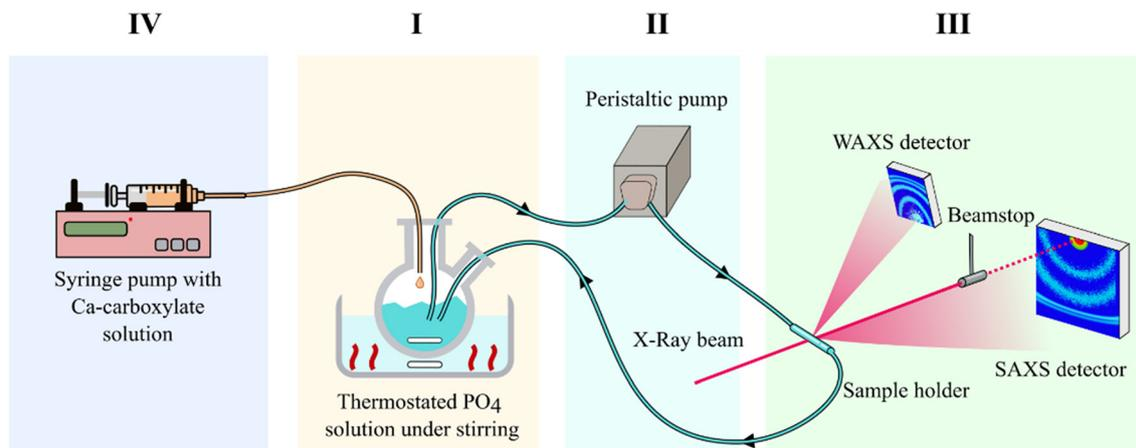
**Fig. 1** Schematic representation of the setup employed for real-time *in situ* SAXS/WAXS measurements during the formation of HA nanoparticles. The setup measures SAXS and WAXS simultaneously in the same sample volume. (I) Thermostated reaction vessel with PO<sub>4</sub> solution, (II) peristaltic pump, (III) sample holder and SAXS/WAXS detectors, (IV) Ca solution syringe pump injector.
