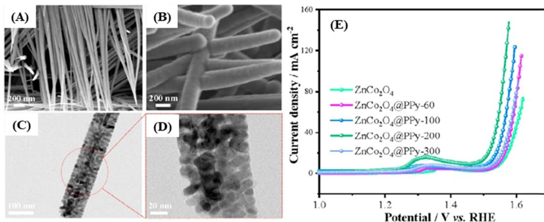
Fig. 21 SEM images of ZnCo<sub>2</sub>O<sub>4</sub> (A) and ZnCo<sub>2</sub>O<sub>4</sub>@PPy-200 (B). TEM images of ZnCo<sub>2</sub>O<sub>4</sub>@PPy-200 (C and D). Linear sweep voltammetry at 2 mV s<sup>-1</sup> for ZnCo<sub>2</sub>O<sub>4</sub> and ZnCo<sub>2</sub>O<sub>4</sub>@PPy samples (E). Reproduced with permission.<sup>275</sup> Copyright © 2021 Elsevier Ltd. All rights reserved.
