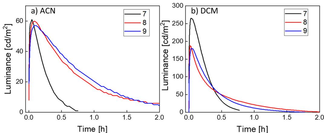
Fig. 5 Time-dependence of the luminance [ $\text{cd m}^{-2}$ ] of LECs ITO/PEDOT:PSS/iTMC:IL(4 : 1)/Al, (iTMC: **7** (black), **8** (red) and **9** (blue)) with the active layer prepared from solutions in ACN (a) and DCM (b). All the devices shown were driven with a pulsed current with an average current density of  $50 \text{ A m}^{-2}$ .
