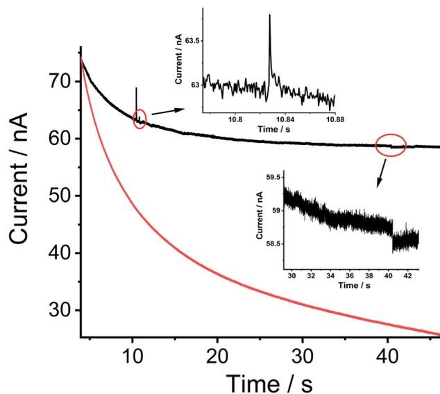
Fig. 6 Chronoamperograms of a carbon micro-disc electrode ( $d = 33 \mu\text{m}$ ) immersed in a  $0.1 \text{ M KNO}_3$  ( $\text{pH} = 6.4$ ) solution containing MWCNTs-NH<sub>2</sub> (black line) or not (red line) at a potential of  $1.90 \text{ V vs. SCE}$ . The inset is an enlarged view of impact spike and step at  $1.90 \text{ V}$  in the presence of MWCNTs-NH<sub>2</sub>.
