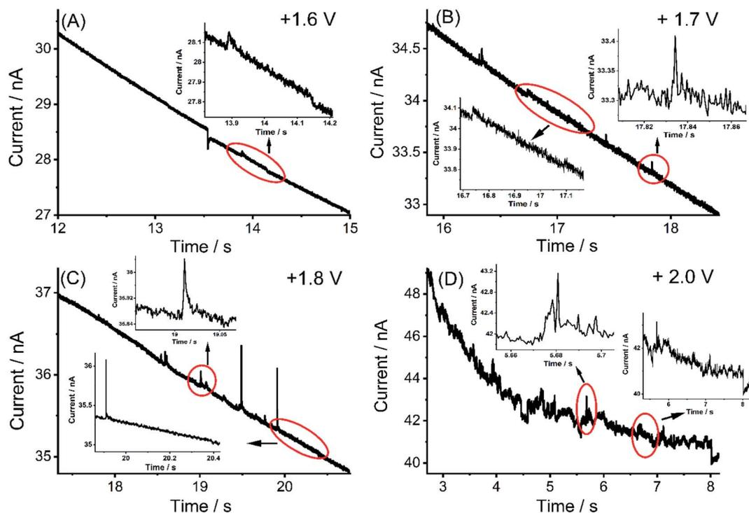
Fig. 3 (A)–(D) Examples of representative chronoamperometric profiles of nano-impact at different potentials (1.60, 1.70, 1.80 and 2.00) in a 0.1 M  $\text{KNO}_3$  (pH = 6.4) solution containing  $0.01 \text{ g L}^{-1}$  MWCNTs. No spikes or steps were detected below/at 1.50 V.
