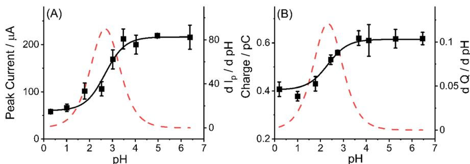
Fig. 8 (A) Relationship between oxidative peak current of MWCNTs-NH<sub>2</sub> modified GCE and pH value of solution; (B) relationship between average charge of oxidative spikes and pH value of solutions in the presence MWCNTs-NH<sub>2</sub> (black square: experimental data; black solid line: simulated curve, and red dotted line: differential curve of experimental data).
